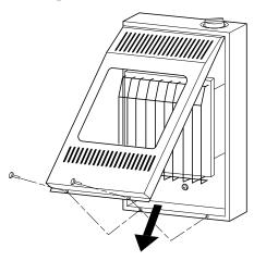
Figure 8 - Removing Front Panel Of Heater
